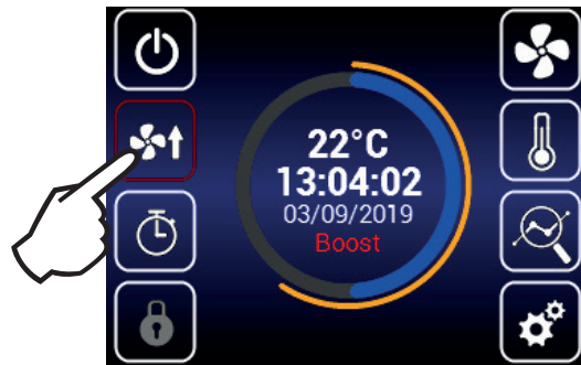
The BOOST mode is activated by touching symbol BOOST regime is displayed in ventilation mode area
