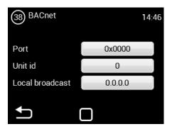
The BACnet menu is used to set the unit's network communication (ModBus TCP).
