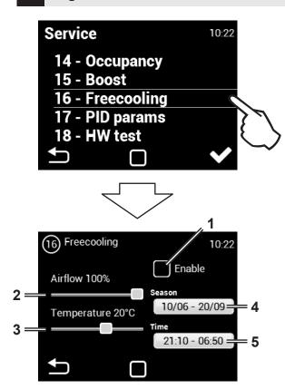
NIGHT VENTILATION is evaluated even if the unit is in Standby mode (at the selected date and time the unit activates and evaluates where night ventilation can be activated - Prefreecooling)
