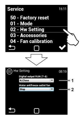
In this menu you can set the logic of using the RUN contact and the logic of antifreeze protection
