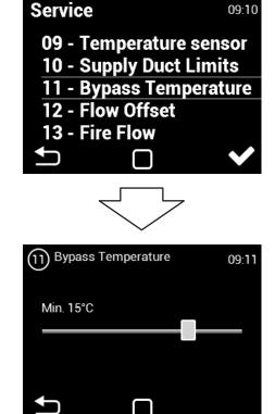
Setting of minimum outdoor temperature from which the bypass opening is allowed (range 0-20°C)
