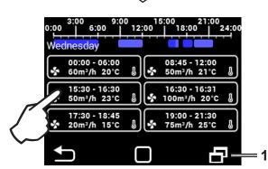
Touch to set individual intervals of ventilation (time ON/OFF, vent. mode, vent. level, temperature)
