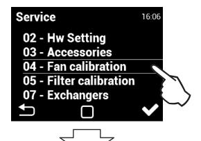
The calibration takes several minutes. Do not disconnect the unit, wait until it's completed. During the calibration the unit determines the maximum pressure loss, when the fan runs at full rate.
