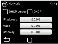
The NETWORK menu serves for setting the network communications of the unit (TCP Modbus).
