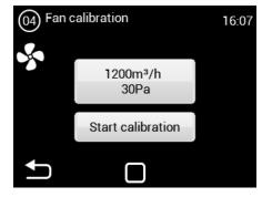
**READ CAREFULLY!** The unit will not work properly if, during calibration, the distribution network is not complete, the flaps or valves are not closed, etc.
