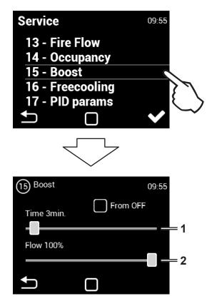
Boost can be activated with the button connected to the input 13/14, or with the Boost button (Fig. Boost) on main screen
