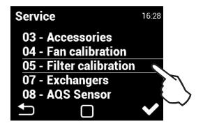
Filter calibration has to be carried out during the first commissioning and after a filter class change.
