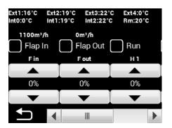
The HW TEST menu is used to test all the connected components and accessories. These parameters are not saved.
