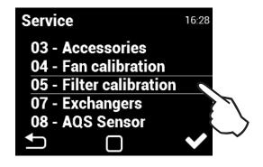
Filter calibration has to be carried out during the first commissioning and after a filter class change.
