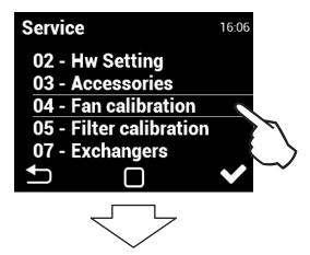
The calibration takes several minutes. Do not disconnect the unit, wait until it's completed. During the calibration the unit determines the maximum pressure loss, when the fan runs at full rate.
