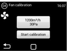
**READ CAREFULLY!** The unit will not work properly if, during calibration, the distribution network is not complete, the flaps or valves are not closed, etc.
