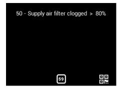
Filter clogging indicator is located on the control display panel.
