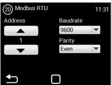
The MODBUS menu is used to set the Modbus communication.
