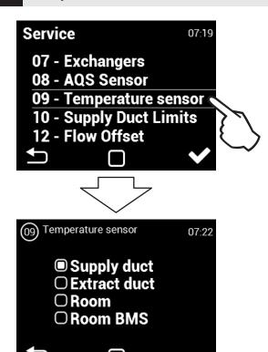
A temperature sensor can be selected to control the air temperature. The values from the selected sensor will be used for temperature control and will be displayed on the main controller screen.
