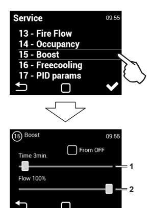
Boost can be activated with the button connected to the input 13/14, or with the Boost button (Fig. Boost) on main screen
