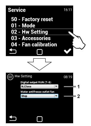
In this menu you can set the logic of using the RUN contact and the logic of antifreeze protection  $\,$
