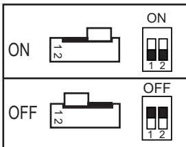
Jumper position PCB
